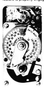
Turn key counter-clockwise until the desired locking time is directly opposite the pointer on the time movement dial. Repeat this step for each movement in the lock. Each mark on the dial corresponds to one hour while each audible "click" represents 12 minutes.
