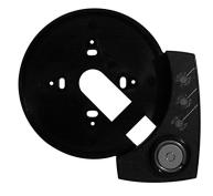
Keypad Extension Base — Installed under the keypad. This is required when using the lock's Service Mode operation or audit trail function. The extension base provides a green LED to indicate "Status 1", and a red LED to indicate "Status 2" and a yellow LED to indicate "Mode" of lock operation. The extension base also provides a port for communication with Touch Keys.
