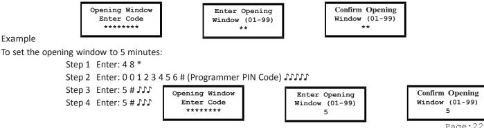
If time delay has not been previously set, the opening window setting may begin immediately upon input of the correct code sequence.
