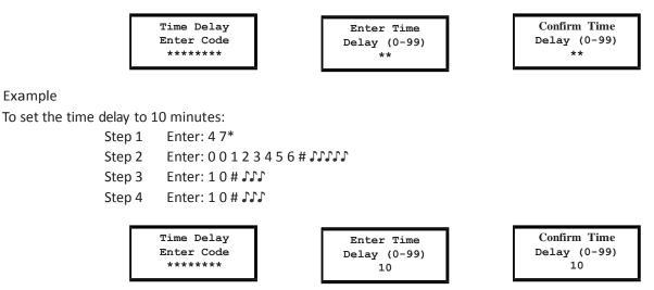
To eliminate the time delay period, enter 0 for the time delay minutes.
