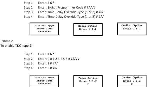
The TDO TYPE 2 function has now been enabled. The code in position 29 can now be used to open the lock without waiting for the time delay countdown.
