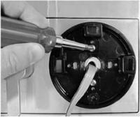
1. Run the connector and wire cable through the center hole of the mounting base. Then use the included 8-32 machine screws to attach the base to the safe door. The attaching screw holes will line up with those used for any standard S&G dial ring (excluding R132 key locking dial rings).
